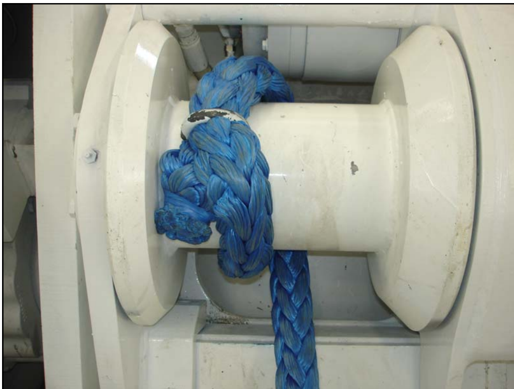
Synthetic Winch Rope clamped by U-bolt
