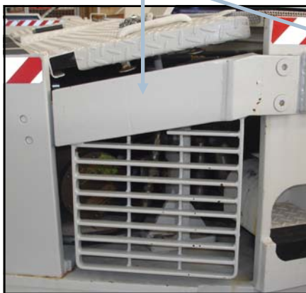
Cooling Fan and Alternator Grills
